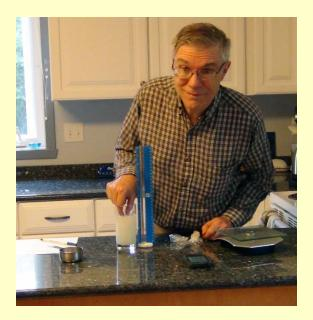
Due to the difficulty in timing the marble fall-time while I was also dropping it and watching when it hit the bottom, I got someone else to run the timer while I dropped the marble and observed when it hit bottom.
